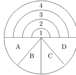
Fig. 3 A wedge-ring detector
