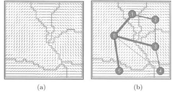
**Fig. 11** Structural features using a relational graph [36]
