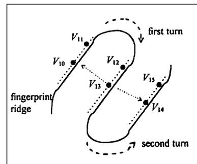
**Fig. 14** The global geometry of a twin loop and features that can be used to recognise it [19]
